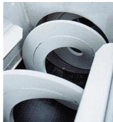
*A section of 480 mm diameter screw and trough.*
